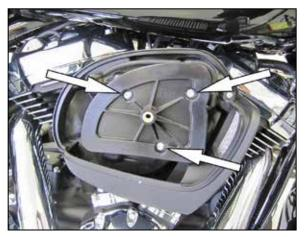
3. Remove the three bolts that secure the air filter element and then remove the air filter and crank case breather tubes.
